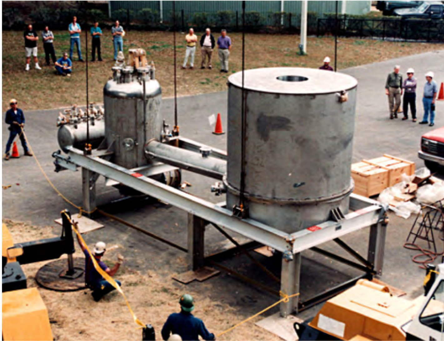
Arrival of 45 T hybrid magnet cryostat at the National High Magnetic Field Laboratory, Florida State University, Tallahassee
