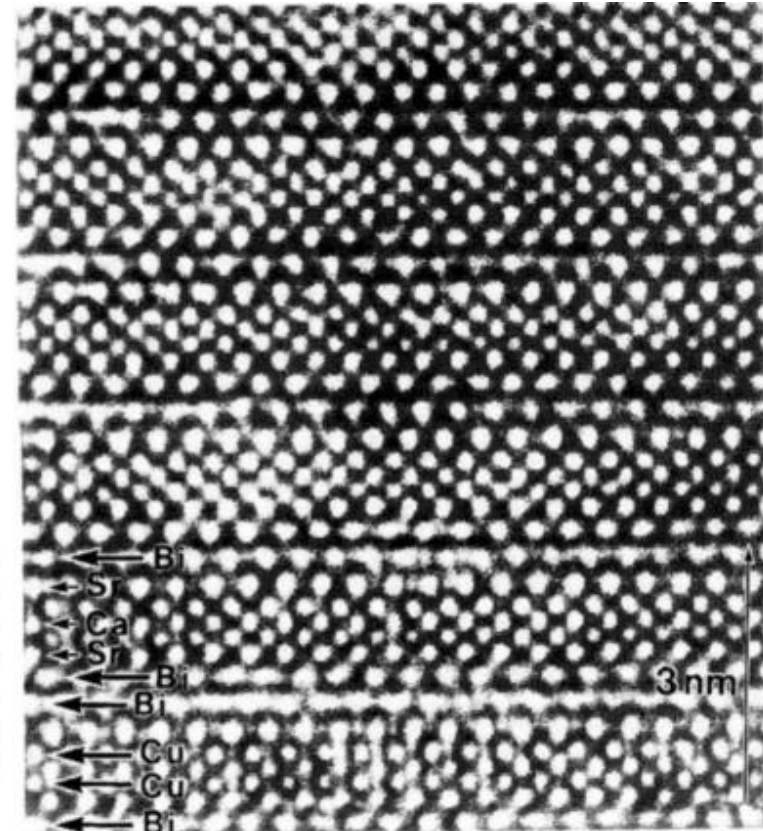
Fig. 10.29. High-resolution transmission electron microscope (TEM) picture of a \text{Bi}_2\text{Sr}_2\text{CaCu}_2\text{O}_{8+x} film. For transmission perpendicular to the c -axis of the crystal the layer structure of the superconductor is visible. Light and dark points correspond to the positions of rows of atoms. (After [10.24].)
