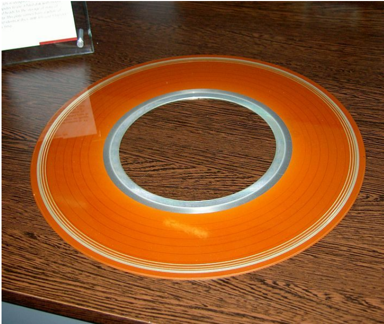
A storage plate Covered with iron oxide
