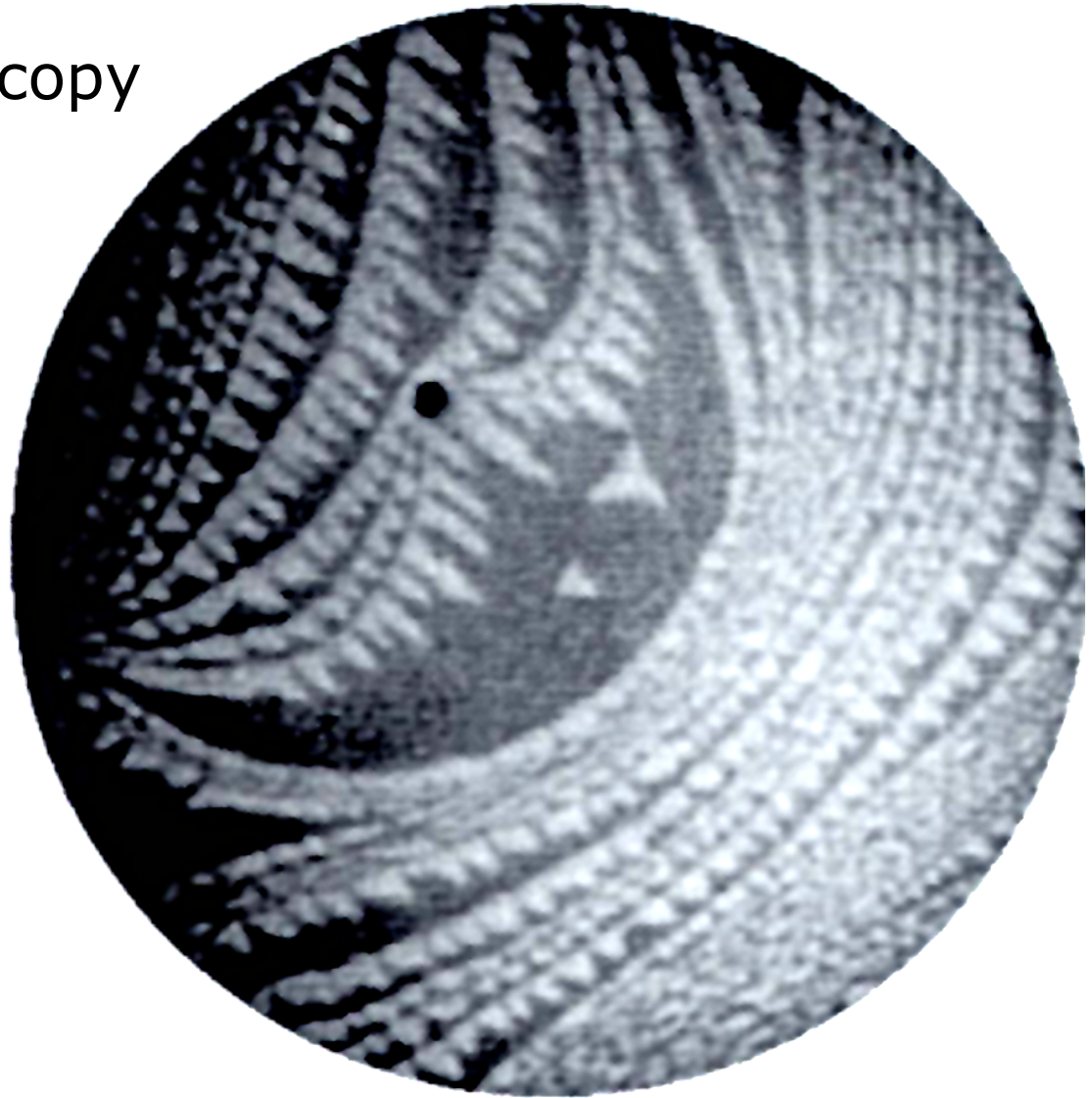
Fig. 7.11. Bright-field LEEM image of the Si(111) 7\times 7 \leftrightarrow 1\times 1 phase transition. The 7\times 7 phase (bright) decorates the atomic steps during the phase transition, while the terraces are mostly covered by the 1\times 1 structure (dark). Contrast is due to the difference in the (0,0) structure factor for the two phases. The field of view is 5 \mu\text{m} (after Tromp [7.7])
