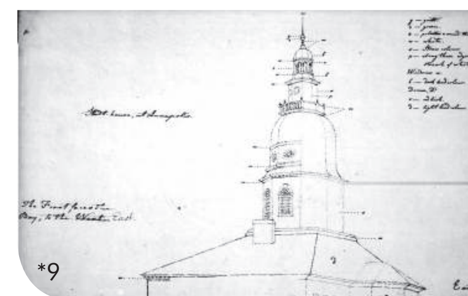
*9 Constructions of lightning rod for the Maryland State House
