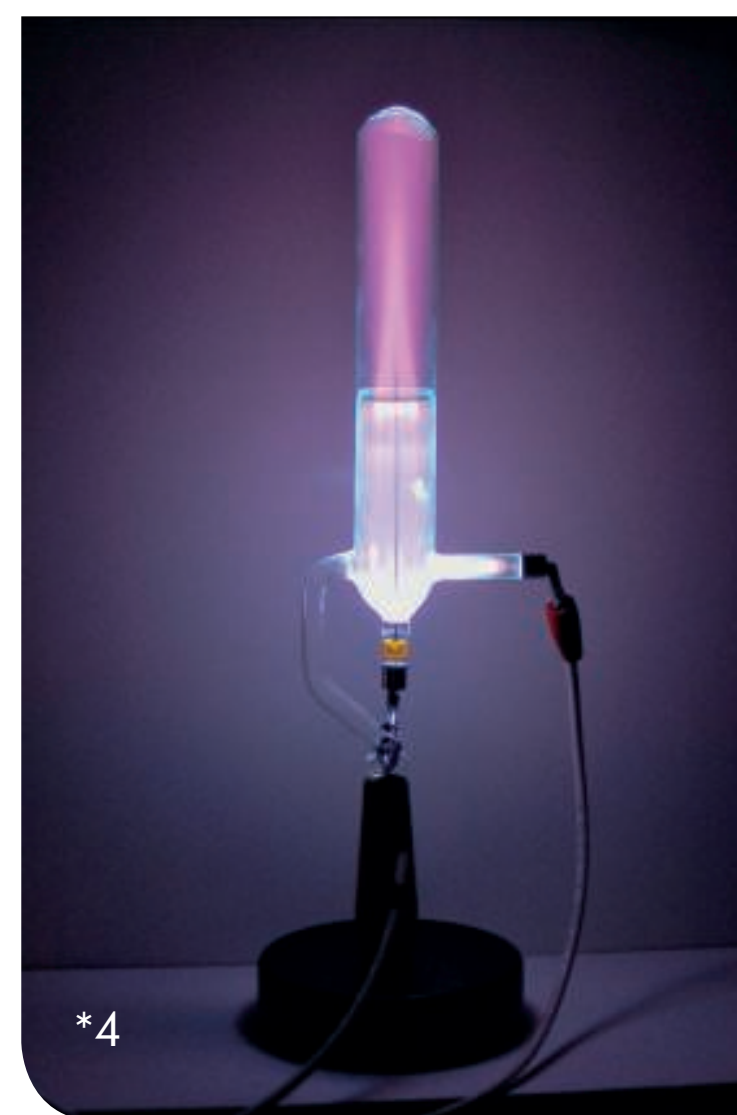
Canal rays observed in a discharge tube
