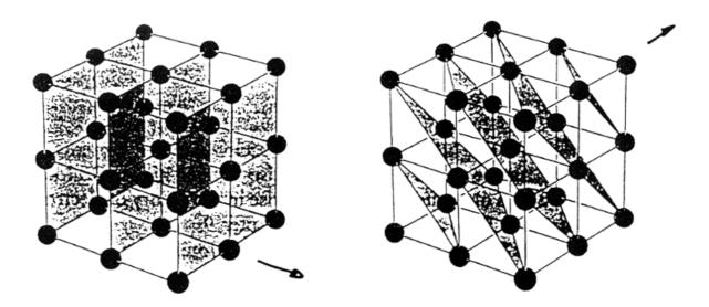
Two ways of representing a simple cubic Bravais lattice as a family of lattice planes (shaded)
