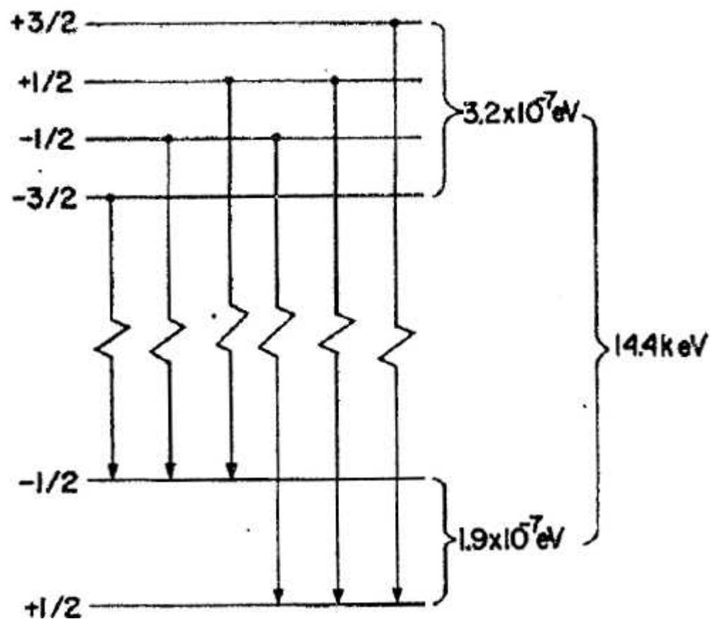
FIG. 1. Zeeman splittings of the two low levels of  $\text{Fe}^{57}$  by the internal magnetic field at the nucleus in ferromagnetic iron. The transitions are those appropriate to magnetic-dipole radiation.
