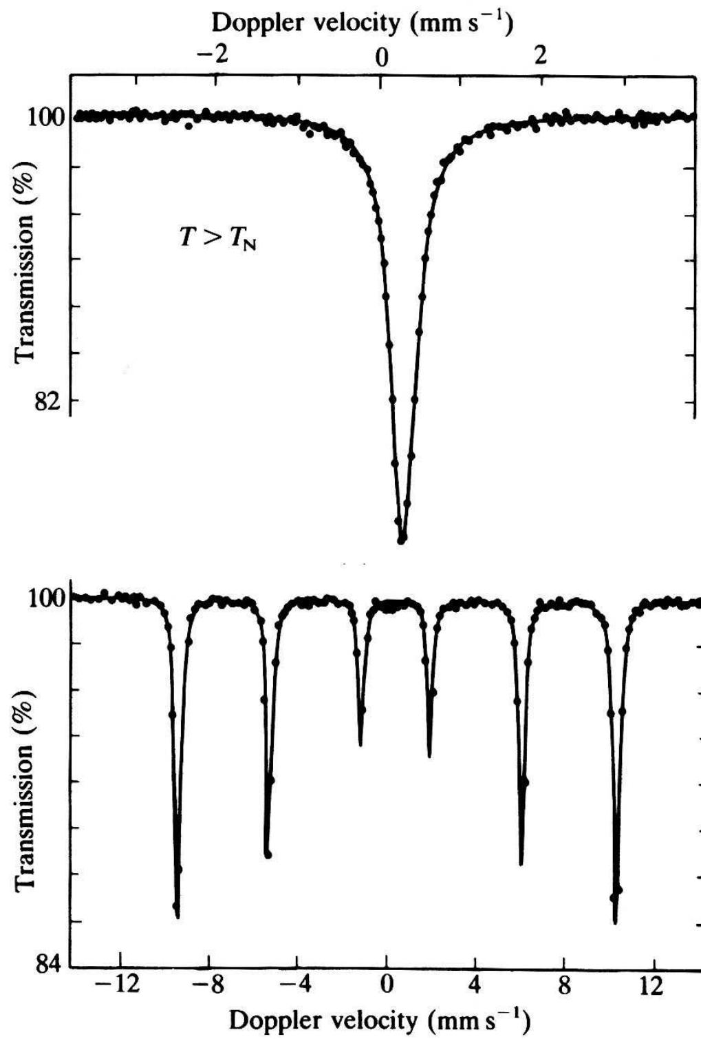
FIG. 4. Typical spectra for metallic  $\text{Fe}^{57}$  between room temperature and the Curie temperature. The single-line source ( $\text{Co}^{57}$  in Cu) was at the temperature of liquid nitrogen.
